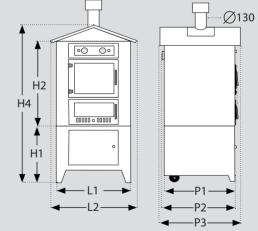
For built-in versions the width corresponds to the dimension **L1**, while the height is given by the dimension **H2** + 50mm of the flue outlet duct
